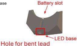
3. Feed the lead that you bent in Step #1 through the hole next to the battery slot
