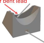
4. Trim excess lead using a wire cutter or flush cutter, leaving enough to bend and tuck the top lead into the battery slot. Repeat this step for the bottom lead, tucking it into the battery slot.
